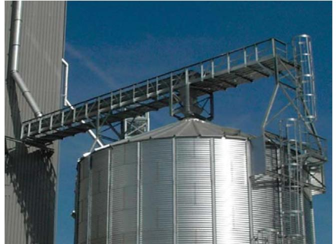
The purpose of the **PETKUS Trough Chain Conveyor TK 400 / TK 520** is the horizontal transport of free flowing, bulky products such as grain, pulses, oilseeds and similar agricultural products.
