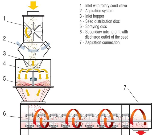
The **PETKUS Chemical Seed Treater CT 10** is used for continuous, wet chemical treating of seed such as grain, corn, pulses etc.
